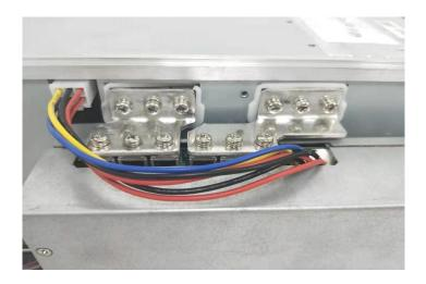
Insert the power 6pin plug into the 6pin socket of the machine as shown below.
